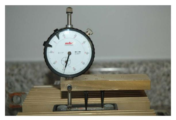
The curvature of the spring can be read from the gauge. If you wish the black pointer can be rotated to this reading for future reference.
